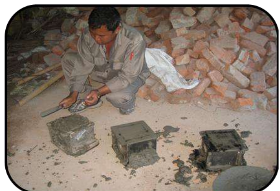
Quality control by testing concrete grade
